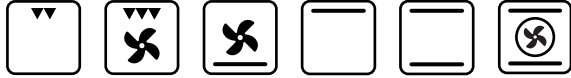
Dual Grill Fan Grill Base Heat with Fan Top Heat Conventional Fan Assist
