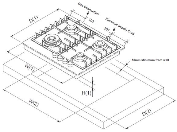
Product dimensions 55mm (H1), 590mm (W1), 510mm (D1) Cut out dimensions 560mm (W2), 480mm (D2)
