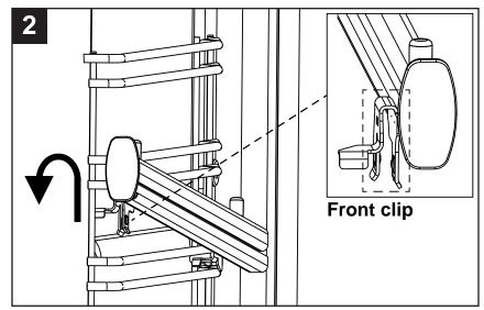
Locate the front clip onto the shelf runner and firmly push the front of the guide down until the front clip is secured into place.
