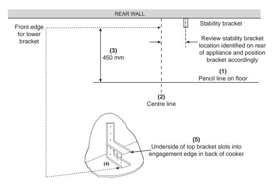
A restraining device shall restrict the appliance movement to no more than 80% of the hose length.
