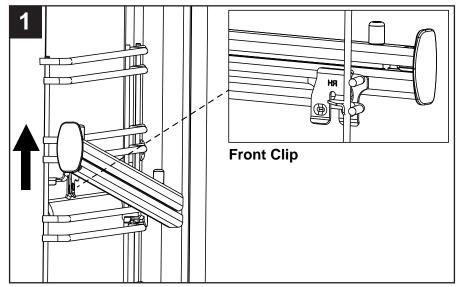
Push the front of the guide upwards firmly, ensuring the front clip is released from the shelf runner.
