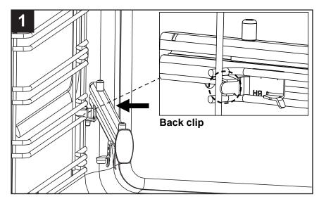
Secure the back clip in between the shelf runner. Ensure the guide is fully pushed back towards the back of shelf runner.
