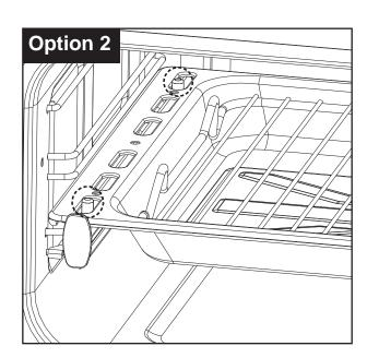
Note: Please ensure the wires / oven pan locate around the small tabs on the telescopic runner.
