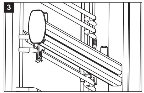
The Telescopic guide should now be fitted correctly and secure to the shelf runner.
