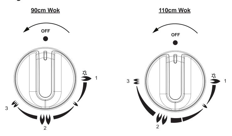
To ignite the outer burner of the wok, turn the control knob to the ignition and flame symbol (1). Hold for 15 seconds until the flame takes hold. Then turn the control knob to the desired power.
