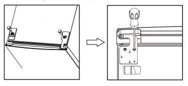
2. Unscrew from the middle hinge by cross screwdriver, then take off the lower door.
