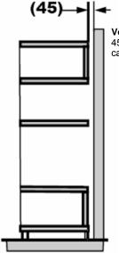
Ventilation: Option 3 (for tower installation)
