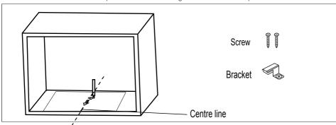
3. Remove the bottom cabinet template and fix the bracket with screw.
