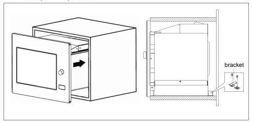
5. Open the door, fix the oven to the cabinet with Screw, at the installation hole.
